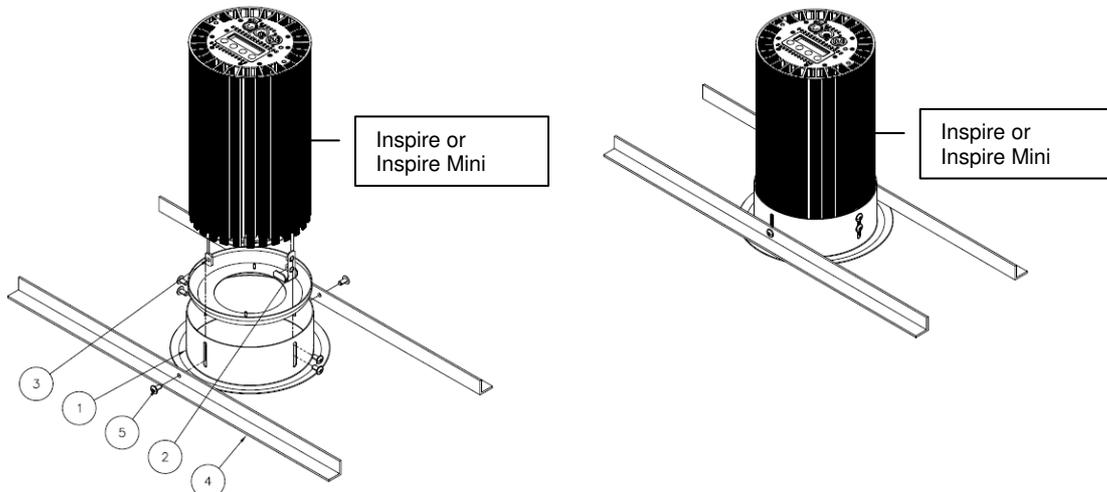
Caution: The angle supports of the ceiling installation kit must be mounted or attached to the ceiling with the appropriate load capacity.
