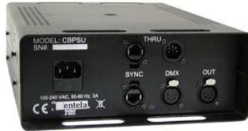
The Color Block PSU-30 delivers power and data via 6 XLR4 outputs. A maximum of five daisy-chained Color Block 2 fixtures can be connected to each XLR4 output. Return lines are not required. The total cable length of each chain must not exceed 60m/200ft. Two in/out ethernet RJ45 connectors are available for synchronisation.
