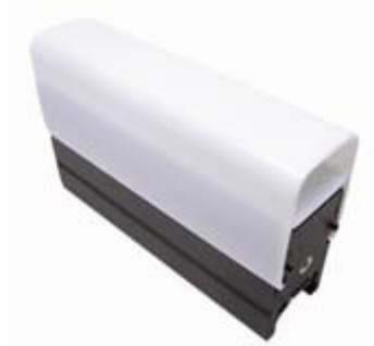
The LED pipe is available in 250mm and 1300mm lengths and simply snaps into the fixing slots on the fixture body. The LED pipe blends and diffuses the RGBA LED output of adjacent cells, taking the resulting colour. The LED pipe is particularly effective at linear colour chase effects.
