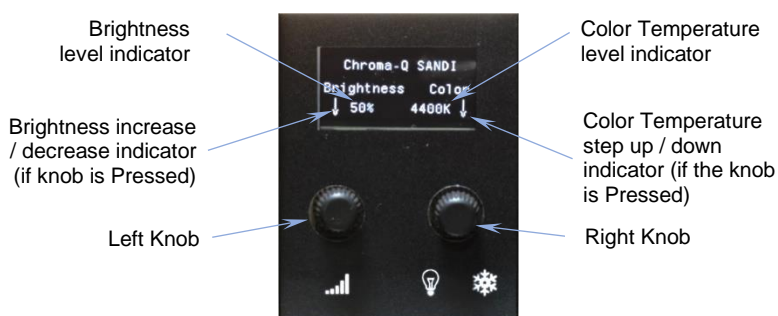
Fig. 2: Front Control Panel (Balanced Idle mode: both sides have same Brightness and CCT)
