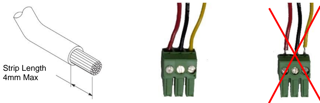
Figure 8: Wire Stripping for Data Connection
