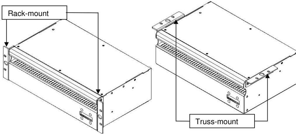
The PSU-300 has a unique Magic Box interlocking enclosure which facilitates easy rack mounting when used in pairs and easy truss mounting via captive nut insert.
