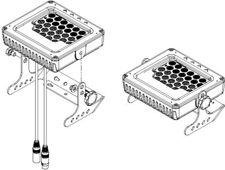
Note: Secure the fixture with a safety bond. A provision for a fixing hold is built into the enclosure.
