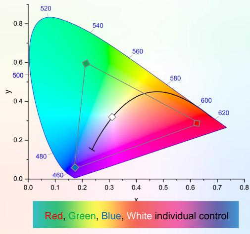
Red, Green, Blue and White control allows for deep saturated colours when needed
