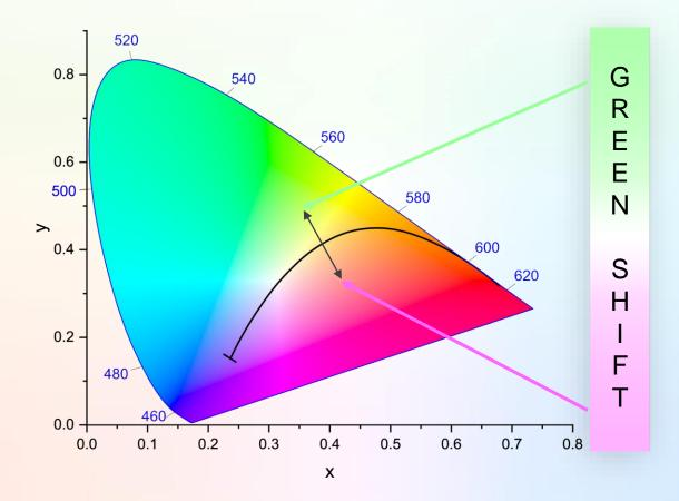
The HUE control allows for a +/- Green shift of 2 between 2800 and 6500K
