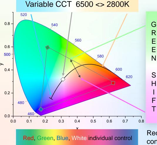
The HUE control allows for a +/- Green shift of 2 between 2800 and 6500K
