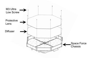
ii. For Space Force onebytwo<sup>™</sup> and twobyfour<sup>™</sup>: Remove the M3x10 Ultra Low Torx Screws from Space Force<sup>™</sup> unit using Torx T6 x 70mm screw driver. Keep them in a secure location. These screws will be used to install the new protective lens.
