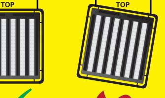
UNIT MUST BE MOUNTED VERTICALLY **SIDE VIEW**
