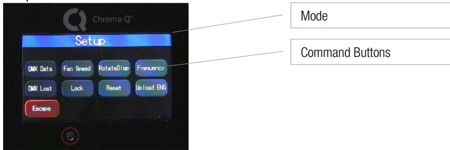
The table shows the fixture setup options available in the Setup screen:
