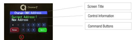
The screen shows the current DMX start address and the new DMX start address. In the screen, the numeric command buttons can be tapped to set the new DMX start address.
