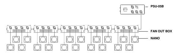
**Power & Data:** Power and control data outputs from the Color Block 2 Plus Nano Fan Out Box is through 4 x RJ45 connections. The total cable length from the Fan Out Box to a fixture must not exceed 3m/10ft.
