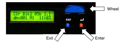
The LCD screen shown above is currently at the Home position and the Main Menu displays the product name and model, software version, current DMX address, current control mode and time.
