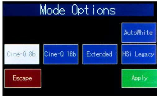
**AutoWhite** When using Cine-Q Mode, it is possible to have the white in RGBW to be automatically adjusted based on the level of Red, Green and Blue in the mix. Additionally, when AutoWhite is enabled, the white channel becomes an inhibitive control of the white level. This means if the White channel is at 0 no white is added to the mix. If at 255, a maximum of white is added based on R,G,B levels
