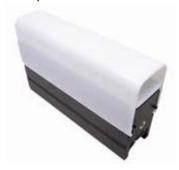
The LED pipe is available in 250mm and 1300mm lengths and simply snaps into the fixing slots on the fixture body. The LED pipe blends and diffuses the RGBA LED output of adjacent cells, taking the resulting colour. The LED pipe is particularly effective at linear colour chase effects.
