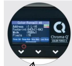
Silk screened arrows near the touch screen should point towards the cyc or wall.
