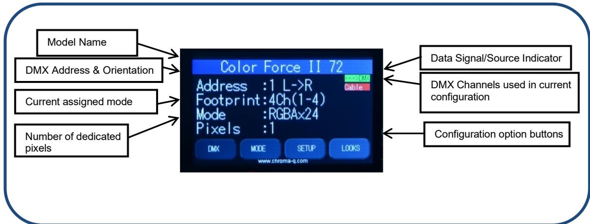
Once the unit is powered up, the display shows the Main Menu with:
