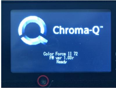
During the short time while the fixture powers on, you can see the fixture type and firmware version. The firmware version is also viewable from the Setup Menu.
