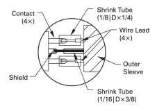
Detail of connector wiring (typical)
