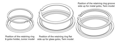
When replacing the retaining rings, start by inserting one end of the ring into the holder and then work around pushing the rest of the ring into its slot in the holder. Check the rings are fully seated in their slots before operating the unit.
