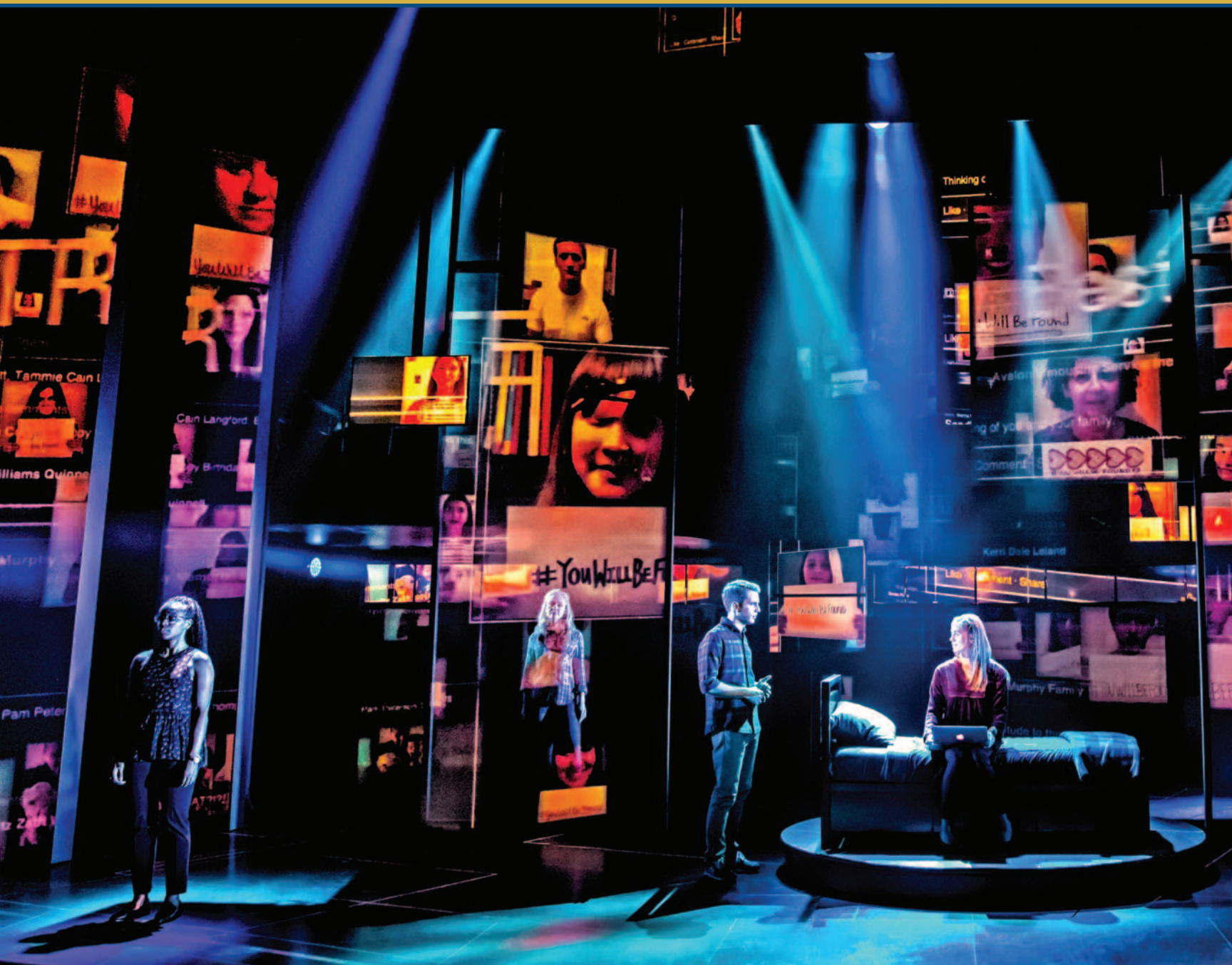
The above image shows the integration of the design’s visual elements. A wagon at stage center suggests a bedroom. Surrounding it are tracking panels and LCD panels loaded with content. Lighting picks out the characters, allowing them to stand out.
