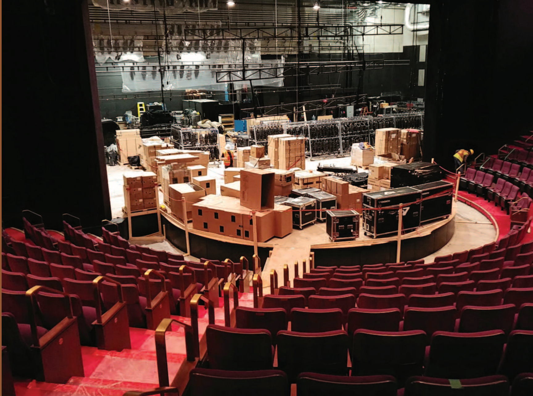
The 797-seat Babs Asper Theatre is convertible from a thrust to a proscenium stage. Because the proscenium opening can be widened or narrowed to accommodate various production designs, the left and right loudspeaker line arrays are designed to travel 8' laterally on custom-designed rigging.
